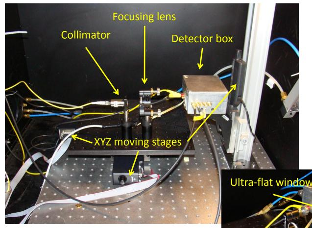
The setup is enclosed in a shielding cabinet, provided with feed-throughs for dry air, water, fibers and signal/bias lines.
