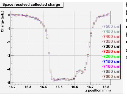
•Collected charge profile is not depending heavily on longitudinal focusing of the laser (almost collimated beam in a region of > 0.5 mm)
