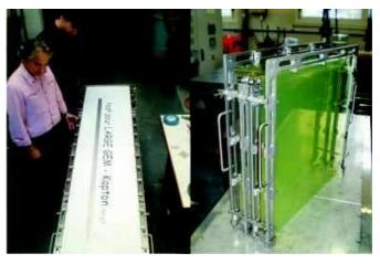
**Figure 10**. Stainless steel portfolio for handling GEMs of up to  $0.5 \times 2 \,\mathrm{m}^2$  during fabrication. Left in the opened state, as it will be when a foil is mounted or dismounted. Right in the folded state, as it will be when it is moved or immersed in chemistry.
