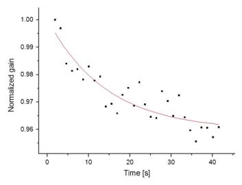
**Fig. 5.** Normalized gas gain of a single mask double GEM stack as a function of time.
