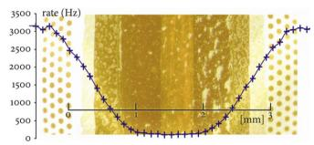
Fig. 6. Microscope picture of the seam and rate scan with the collimated X-ray heam
