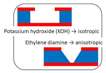
Fig. 1. Polyimide etching using different chemistries.
