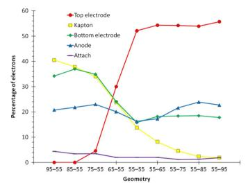
**Fig. 8.** Electron end point distributions. The horizontal axis represents the geometry (hole diameters on the top and on the bottom, in  $\mu$ m), while the vertical axis is the percentage of electrons ending up on each GEM layer.
