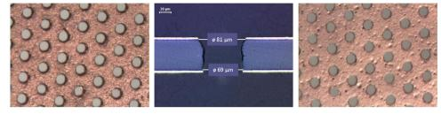
Fig. 3. GEM holes obtained from single mask photolithography, with electrochemical protection and polyimide post-etching. From left to right: top electrode, cross-section, bottom electrode.
