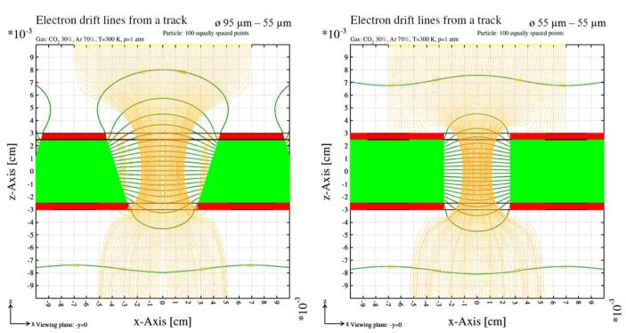
Fig. 7. Simulated equipotential lines and field lines. The hole diameters are  $95 \, \mu m$  in the top and  $55 \, \mu m$  in the bottom layer for the left part, and  $55 \, \mu m$  in both layers for the right part of the figure.
