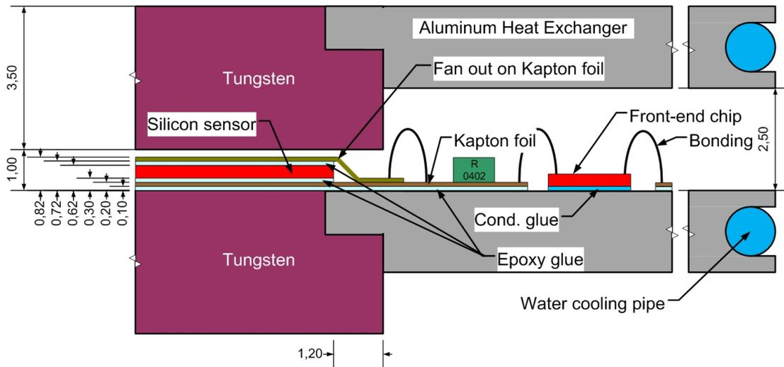
Fig. 6. Cross section showing fan out connections to the front end electronics chips.
