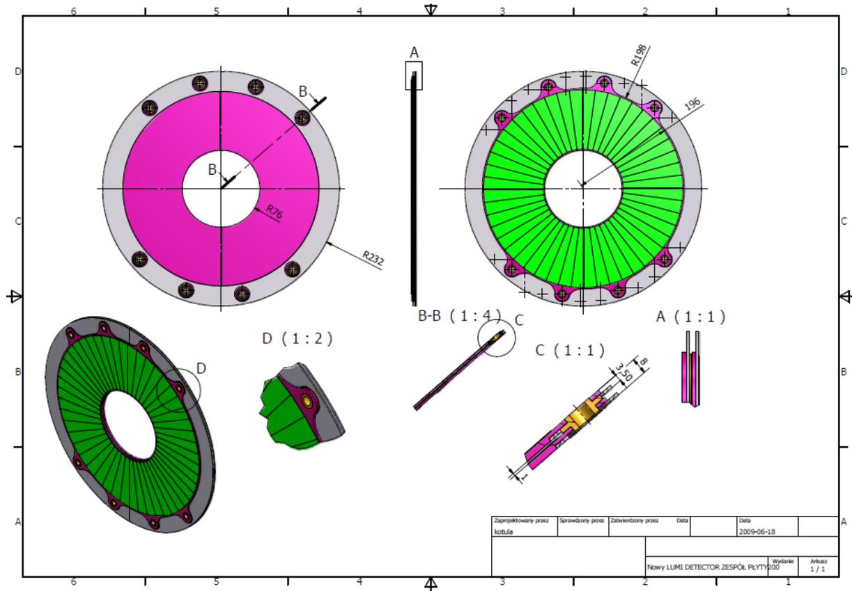
Fig. 3. Tungsten plate with silicon sensors.
