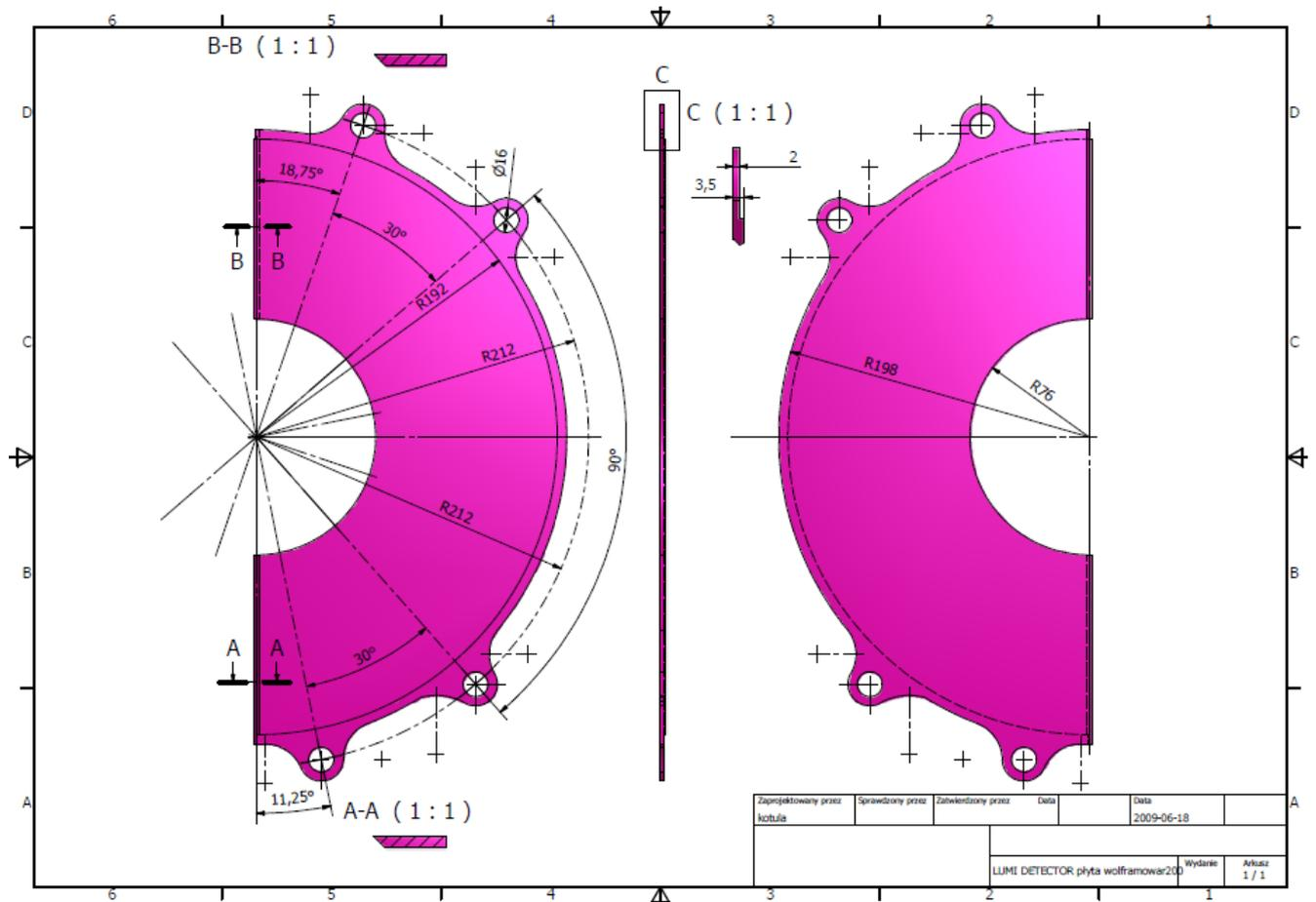
Fig. 2. One tungsten plane with new dimensions.
