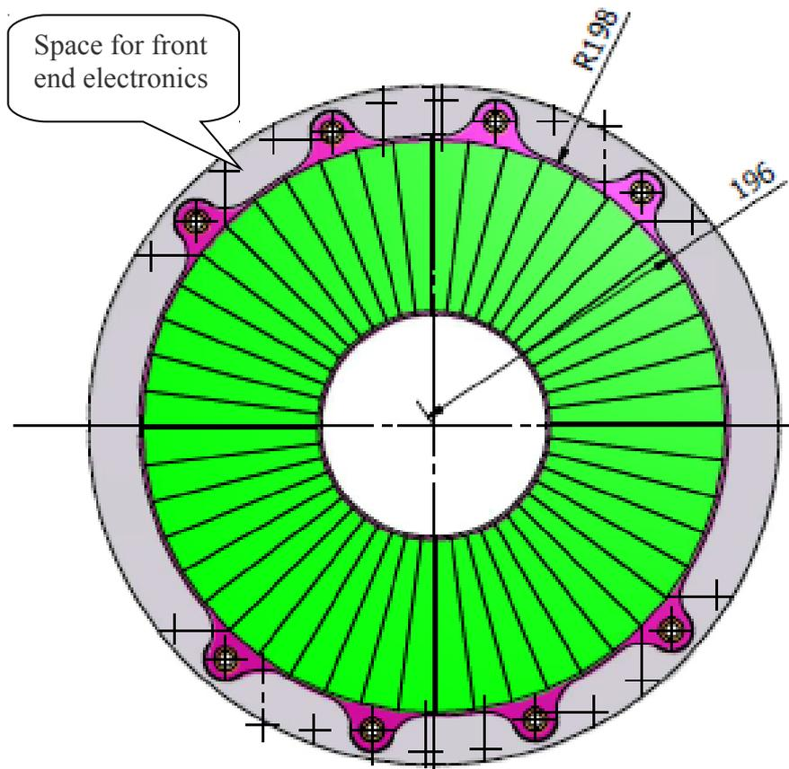
Fig. 5. Space for front end electronics on one half plane.
