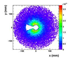
Figure 7: The fluence of neutrons per  $mm^2$  and year crossing a sensor of BeamCal near the shower maximum using the cascade model of Bertini.
