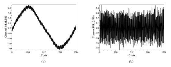
Figure 26: Results of (a) the INL and (b) the DNL errors using 2 fF unit capacitors.
