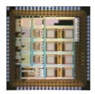
Figure 25: BeamCal Instrumentation ASIC Prototype
