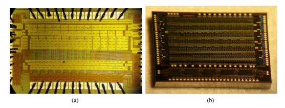
Figure 18: Photograph of prototypes of the front-end ASIC (a) and the ADC ASIC (b)
