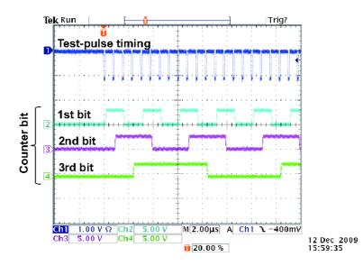
Figure 28: Output signals from the counter block. The lower 3 bits of the 8-bit counter are shown. The test-pulse timing corresponds to the bunch crossing frequency if the ILC.
