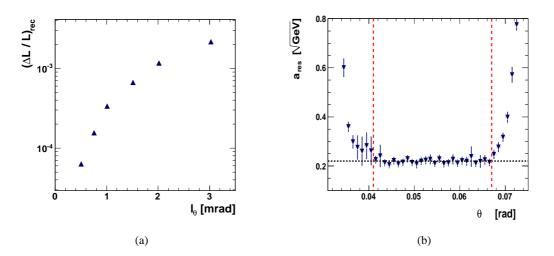
Figure 3: (a) Dependence of  $(\Delta L/L)_{rec}$ , as defined in eqn. (2.3), on the polar angle pad size,  $l_{\theta}$ . (b) The energy resolution,  $a_{res}$ , for 250 GeV electrons as a function of the polar angle,  $\theta$ , covering the polar angle range of the LumiCal.
