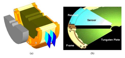
Figure 9: (a) A half-cylinder of BeamCal. The brown block is the tungsten absorber structure interspersed with sensor layers. The orange structure represents the mechanical frame. The blue segments at the outer radius indicate the front-end electronics. In front of the calorimeter a graphite shield, shown in grey, reduces the amount of low energy particles back-scattered into the tracking detectors. (b) A half-layer of an absorber disk assembled with a sensor sector and the front-end readout.
