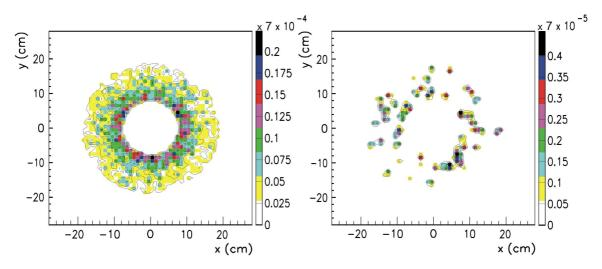
Figure 12: Average number of hits originating from four-fermion interactions per bunch crossing on the first plane of LumiCal at 500 GeV, before (left) and after (right) application of Bhabha event selection criteria.
