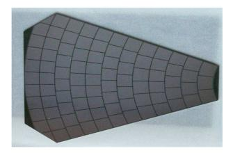
Figure 14: A prototype of a GaAs sensor sector for BeamCal with pads of about 30 mm<sup>2</sup> area.
