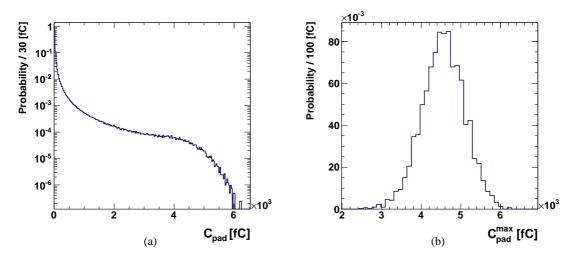
Figure 4: (a) Normalised distribution of the charge deposited in a detector pad,  $C_{pad}$ , by 250 GeV electron showers. (b) Normalised distribution of the maximal charge collected in a single pad per shower,  $C_{pad}^{max}$ , for 250 GeV electron showers.
