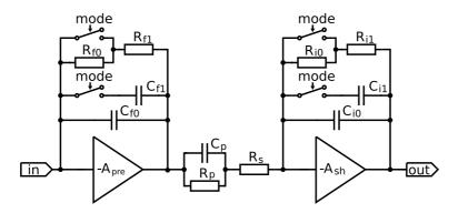
Figure 19: Block diagram of the single front-end channel
