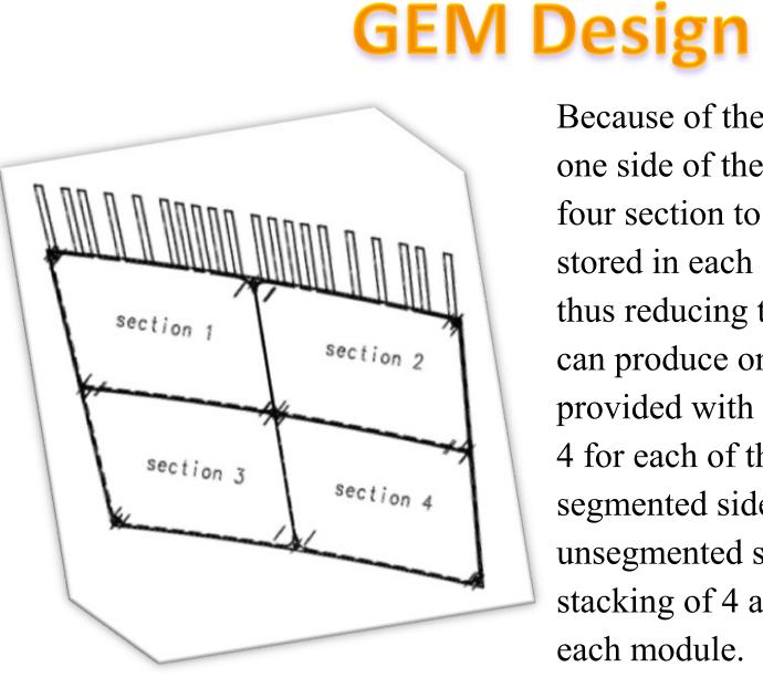
Because of the size of the module one side of the GEM is segmented in four section to reduce the energy stored in each capacitive structure thus reducing the damage a discharge can produce on them. Each GEM is provided with 20 electrical contacts, 4 for each of the sections on the segmented side and 4 for the unsegmented side, to allow the stacking of 4 amplification stages in each module.
