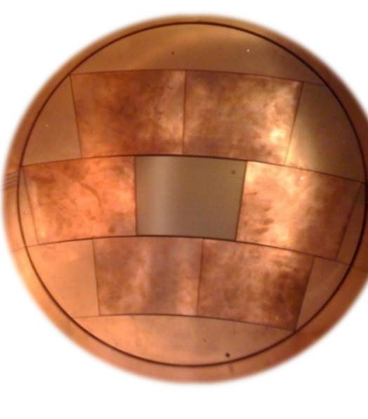
The Gas Amplification and Readout stage of the LPTPC is composed of seven modules that can be equipped with different devices. This prototype has been used to test both G.E.M. and MICROMEGAS amplification systems with pad or pixel readout
