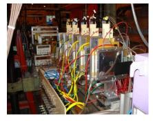
**Fig. 16:** Experimental setup of several resistive bulk Micromegas detectors in the MAMMA beam facility.
