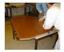
Fig. 17: Large size bulk Micromegas prototype for ATLAS muon system upgrade.
