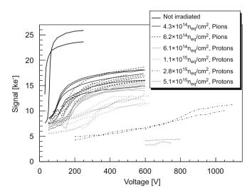
**Fig. 2.** Most probable signal from single pixel clusters as a function of the sensor bias. Each line represents one sample.
