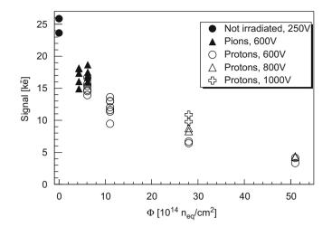
Fig. 3. Most probable signal as a function of the irradiation fluence.
