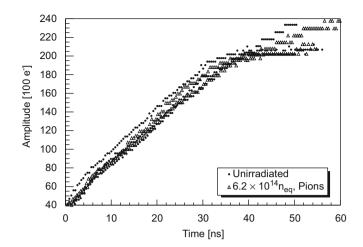
**Fig. 5.** Pulse shape of an injected test signal measured in one pixel of three unirradiated ROCs and two ROCs irradiated to  $6.2 \times 10^{14} n_{eo}/cm^2$ .
