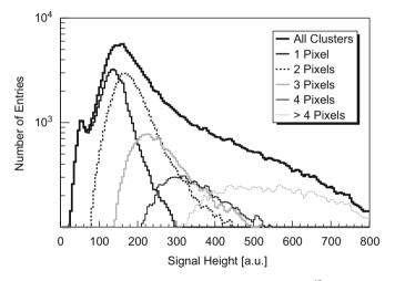
**Fig. 1.** Pulse height distribution of a sample irradiated to  $2.8 \times 10^{15} n_{eq}/cm^2$  at a bias voltage of 800 V in arbitrary units (1 unit corresponds to about 65 electrons).
