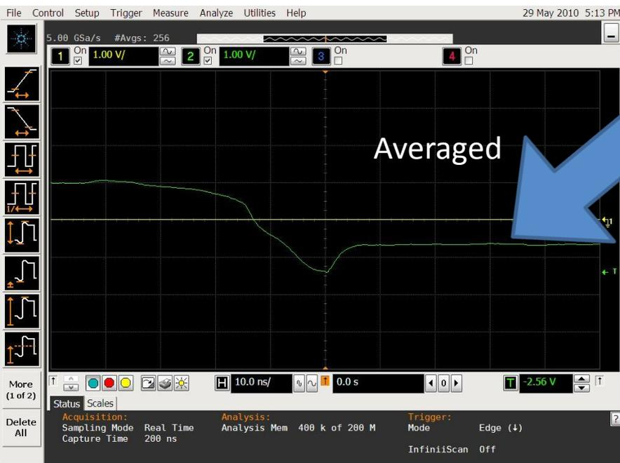
*(Microdischarges in  $1.7e14$  p irradiated sample at 700 V)*
