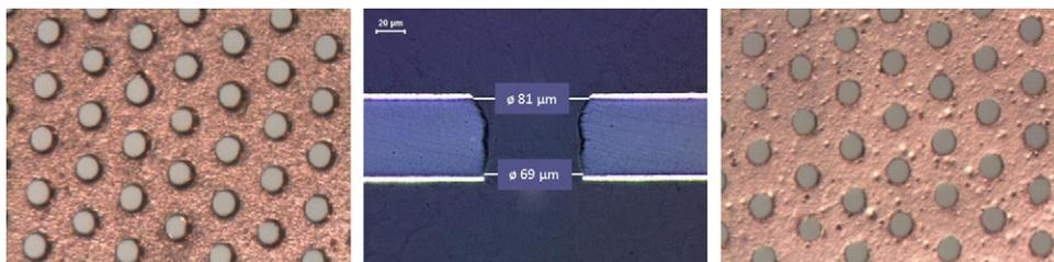
**Fig. 3.** GEM holes obtained from single mask photolithography, with electrochemical protection and polyimide post-etching. From left to right: top electrode, cross-section, bottom electrode.
