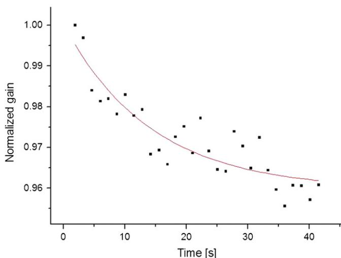
**Fig. 5.** Normalized gas gain of a single mask double GEM stack as a function of time.
