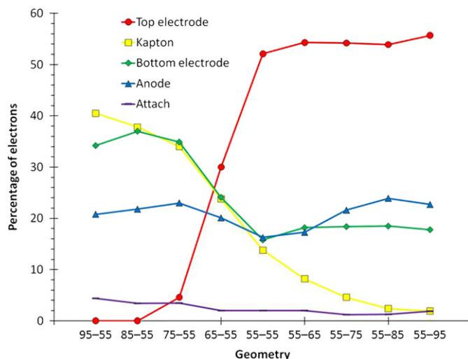
Fig. 8. Electron end point distributions. The horizontal axis represents the geometry (hole diameters on the top and on the bottom, in  $\mu\text{m}$ ), while the vertical axis is the percentage of electrons ending up on each GEM layer.
