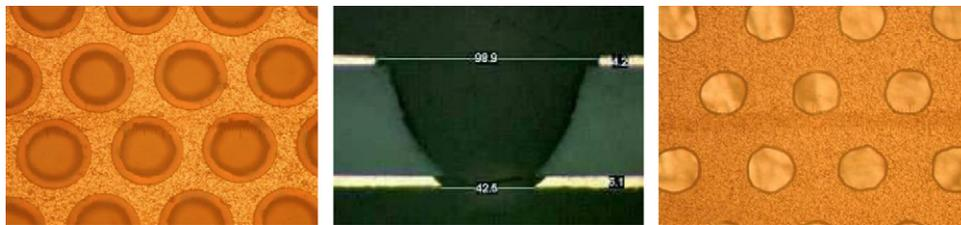
**Fig. 2.** GEM holes obtained from single mask photolithography. The left picture shows the top copper electrode, where the rim is visible, while the right picture shows the bottom layer. The central picture is a hole cross-section.
