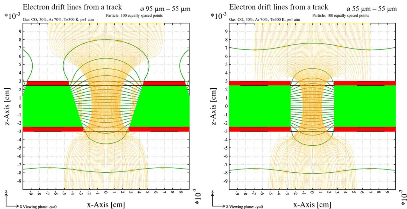
Fig. 7. Simulated equipotential lines and field lines. The hole diameters are 95  $\mu\text{m}$  in the top and 55  $\mu\text{m}$  in the bottom layer for the left part, and 55  $\mu\text{m}$  in both layers for the right part of the figure.
