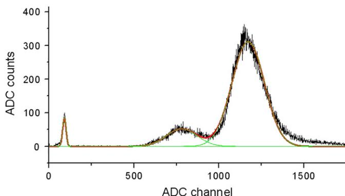
**Fig. 4.** Copper spectrum obtained with a double GEM stack based on single mask GEMs with electrochemical protection.
