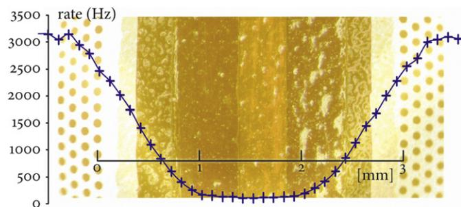
**Fig. 6.** Microscope picture of the seam and rate scan with the collimated X-ray beam.
