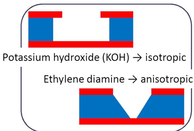
Fig. 1. Polyimide etching using different chemistries.
