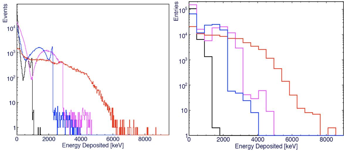
Figure 10. Energy deposition for 10 MeV neutrons in oxygen (blue line), carbon (pink line), argon (black line) and hydrogen (red line) gaseous chambers (1mx1mx1m).
