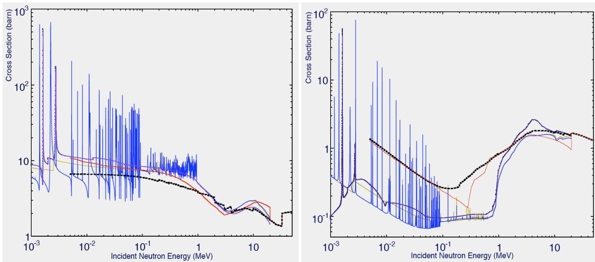
Figure 5. G4NDL is missing xs for Krypton ( $Z=36$ ). Instead, is using Bromine’s ( $Z=35$ ) xs. Geant4 does not follow any of the libraries. Large differences appear in the case of non-elastic interactions. For the case of Krypton, G4NDL needs Krypton’s data for a more reliable comparison.
