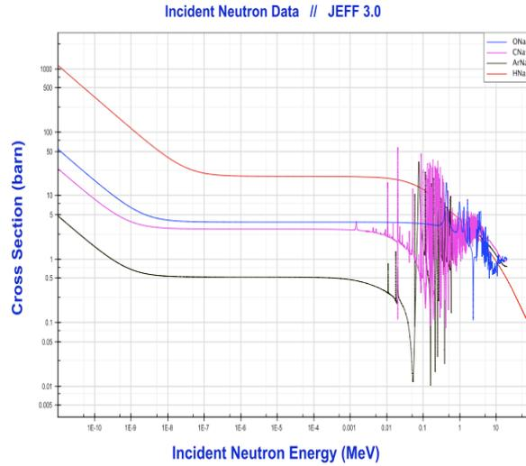
Figure 8. Neutron Cross Section in natural composition of oxygen (blue line), carbon (pink line), argon (black line) and hydrogen (red line).
