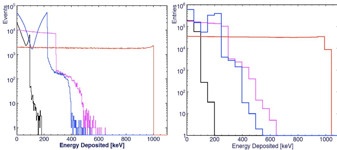
Figure 9. Energy deposition for 1 MeV neutrons in oxygen (blue line), carbon (pink line), argon (black line) and hydrogen (red line) gaseous chambers (1mx1mx1m).
