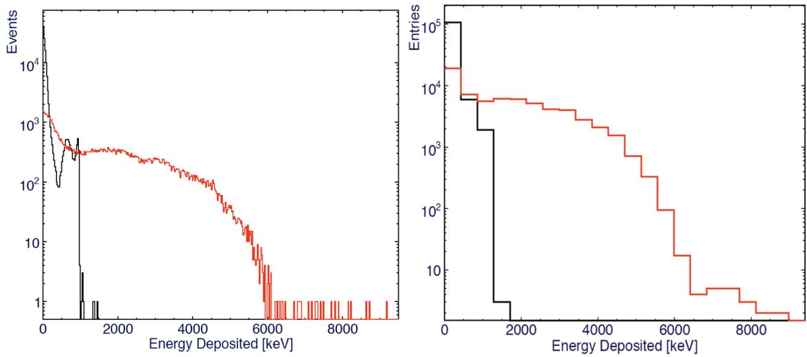
Figure 11. Energy Deposition in 90% argon (black line) (1.782mg/cm<sup>3</sup>) and 10% CH<sub>4</sub> (red line) (0.1782mg/cm<sup>3</sup>) gaseous chambers, for 10 MeV neutrons.
