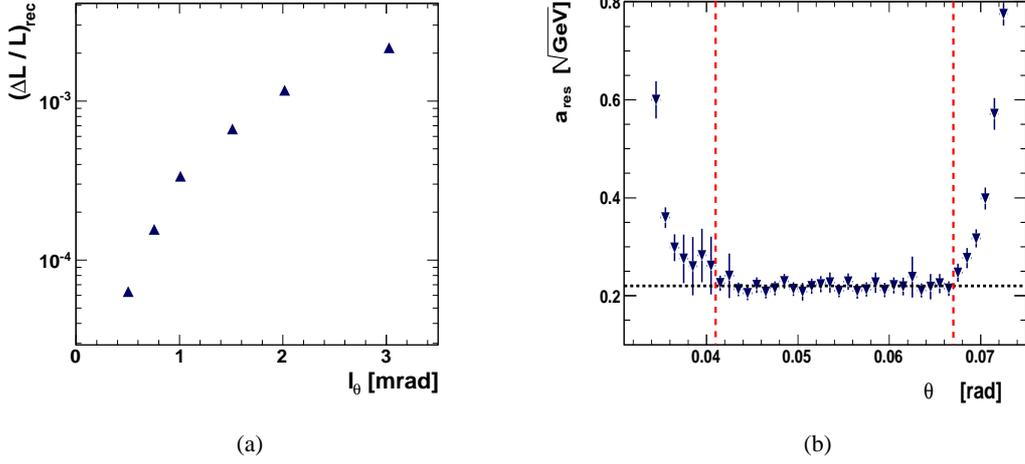
Figure 3: (a) Dependence of  $(\Delta L/L)_{\text{rec}}$ , as defined in eqn. (2.3), on the polar angle pad size,  $l_\theta$ . (b) The energy resolution,  $a_{\text{res}}$ , for 250 GeV electrons as a function of the polar angle,  $\theta$ , covering the polar angle range of the LumiCal.
