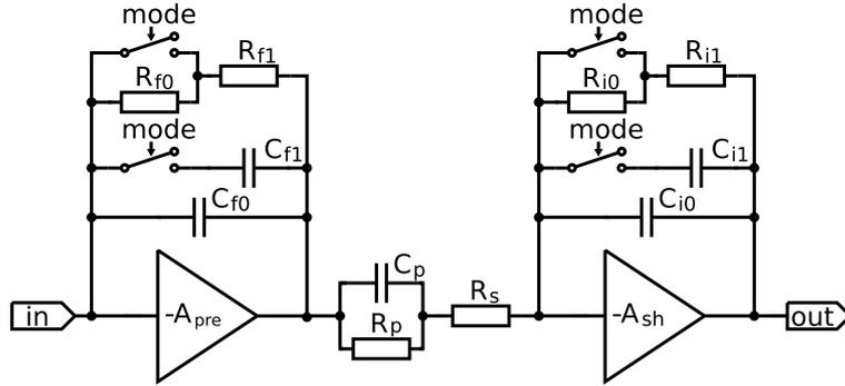
Figure 19: Block diagram of the single front-end channel
