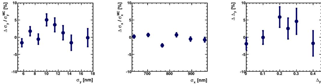
Figure 8: The relative deviations of the vertical,  $\sigma_y$ , and horizontal,  $\sigma_x$ , beam sizes, and the ratio of vertical displacement to the vertical beam size,  $\Delta_y$ , averaged over 50 bunch crossings which are measured by the pair monitor.
