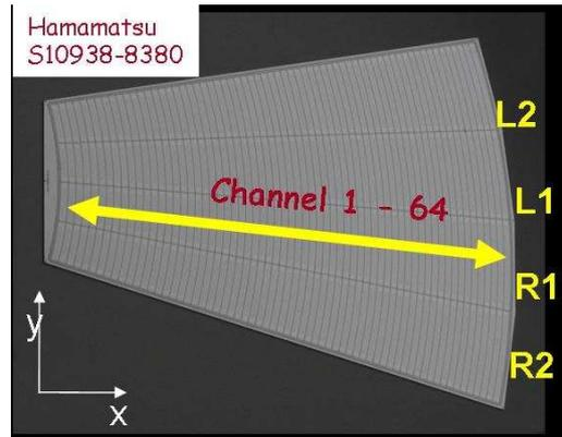
Figure 16: A prototype silicon sensor for LumiCal
