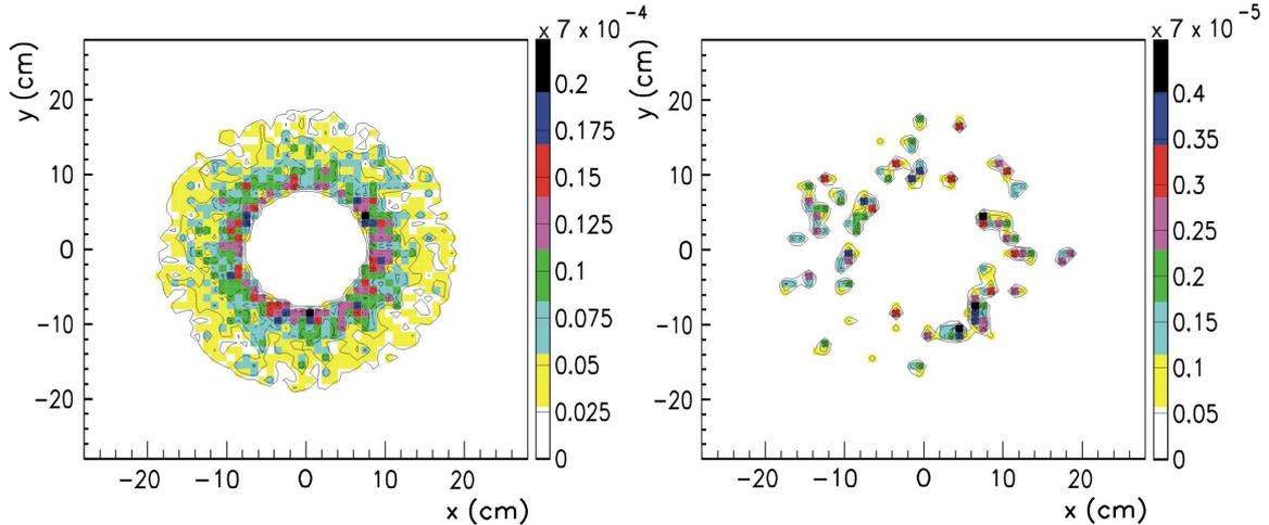
Figure 12: Average number of hits originating from four-fermion interactions per bunch crossing on the first plane of LumiCal at 500 GeV, before (left) and after (right) application of Bhabha event selection criteria.
