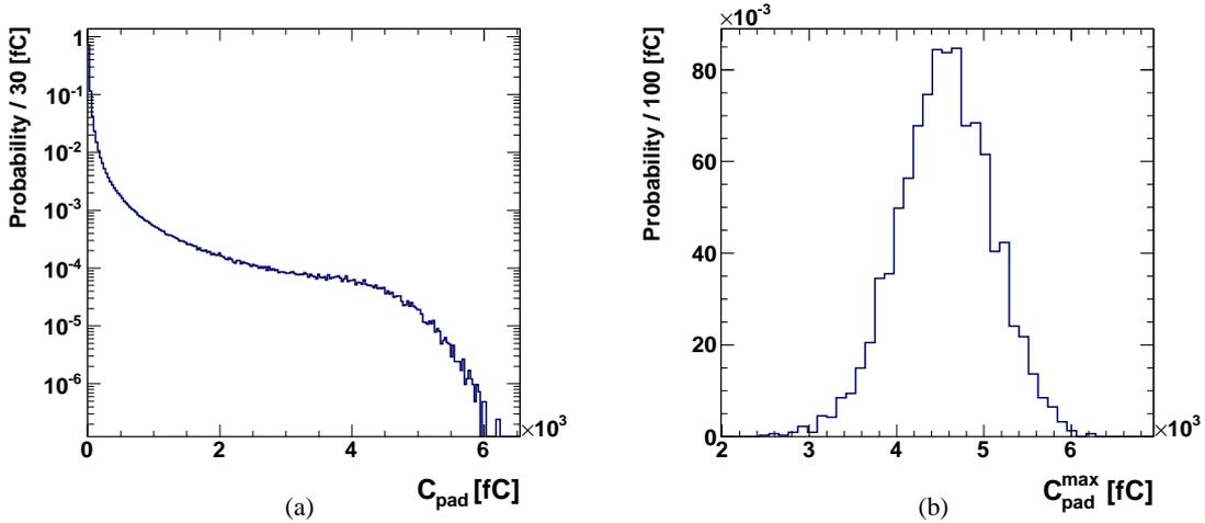
Figure 4: (a) Normalised distribution of the charge deposited in a detector pad,  $C_{\text{pad}}$ , by 250 GeV electron showers. (b) Normalised distribution of the maximal charge collected in a single pad per shower,  $C_{\text{pad}}^{\text{max}}$ , for 250 GeV electron showers.
