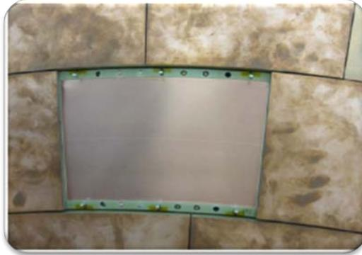
Standard GEM frames made of GRP (Glass Reinforced Plastic)
