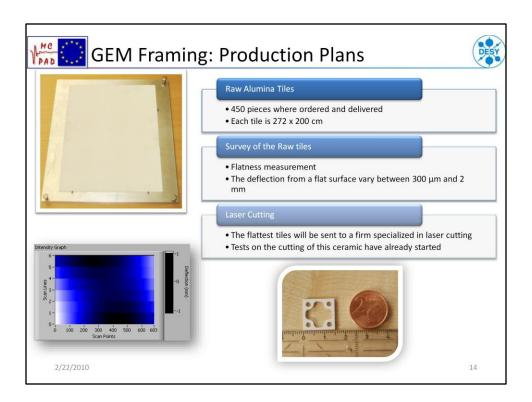
To produce these frames we bought 450 raw tiles and, after a survey of the flatness we are going to laser cut them into the due shape
