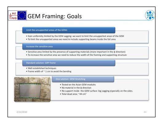
One of the most important features of our design is the GEM framing structure. Our goal in the development of this element of our project was to create a structure which can support and frame the GEM, increasing the sensitive area, reducing the dead space and the amount of material used and supporting as much of the GEM area as possible, keeping that flat and stable
