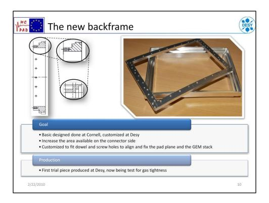
The backframe of the LP modules was designed at Cornell with the Endplate that hosts them. We customized this design to increase the available area on the connector side, as you can see from the left hand side picture where I have emphasized the major changes we made to the original designed. Moreover we added screw and dowel holes to fix and align all the element of the module, backframe, pad plane and framed GEMs
