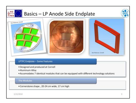
The anode endplate of the LP has been designe at Cornell by Dan Peterson and features seven holes for seven identical modules that can be equipped with the different technologies solutions to be tested. On the left hand side you can see one of the 3d rendering of this device. In the middel picture, on the other hand, you can see this same device built and installed inside the LP equipped with one Micromegas module.
