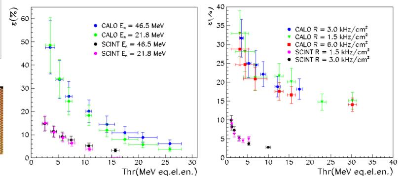
**Very high efficiency, about 4 times larger than what expected** if only the amount of scintillator is taken into account ( $\sim 8\%$  for 8 cm of scintillating fibers)
