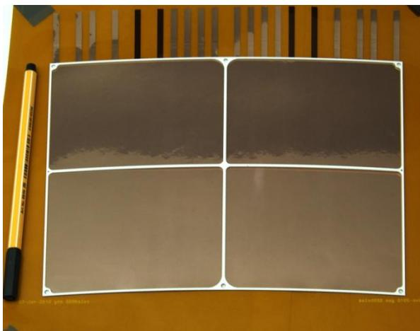
Figure 1: The GEM foil and its ceramic support structure aligned before the gluing.
