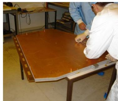
**Fig. 17:** Large size bulk Micromegas prototype for ATLAS muon system upgrade.
