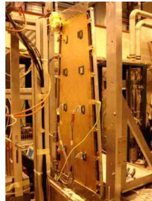
**Fig. 8:** Large area triple GEM detector prototype for CMS muon system upgrade.
