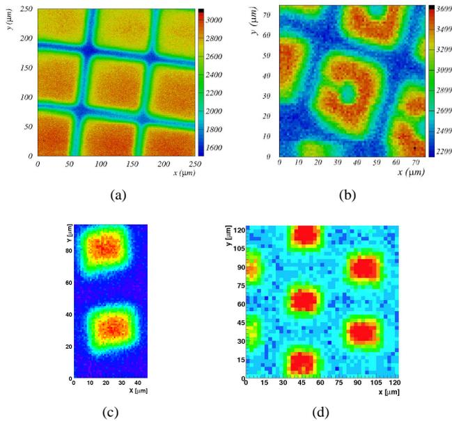
Figure 1: Two-dimensional scans for (a) Hamamatsu H100C, (b) CPTA/Photonique and (c) & (d) STMicronics. Surface scans are valuable to assess the surface sensitivity of SiPM, (a),(b) & (c) were performed with a step size of  $1 \mu\text{m}$  and clearly shows the structure of individual SiPM cells. (d) shows part of a larger surface scan (STMicronics with a step size of  $3 \mu\text{m}$ ) to assess the overall uniformity of the SiPM.
