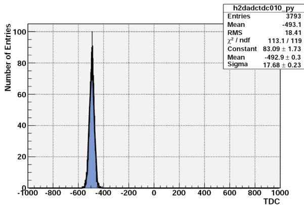
Figure 5: Timing resolution for back-to-back  $\gamma$ 's ( $25 \text{ ps}/\text{bin} \rightarrow \sigma_t \sim 442 \text{ ps}$ ). Hamamatsu  $3 \times 3 \text{ mm}^2$  SiPMs were used for this measurement.
