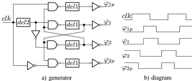
Fig. 6. Block diagram of clock generator and diagram of generated nonoverlapping clocks.
