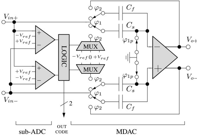
Fig. 3. Simplified schematic of a 1.5-bit stage. Switches set to sampling phase  $\varphi_1$ .
