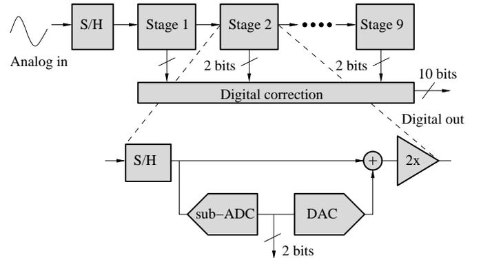
Fig. 1. Pipeline ADC architecture.
