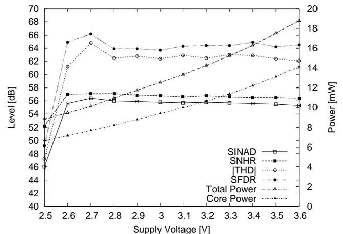
Fig. 14. ADC dynamic performance and power consumption as a function of supply voltage at 10 MHz sampling frequency and around Nyquist input frequency.
