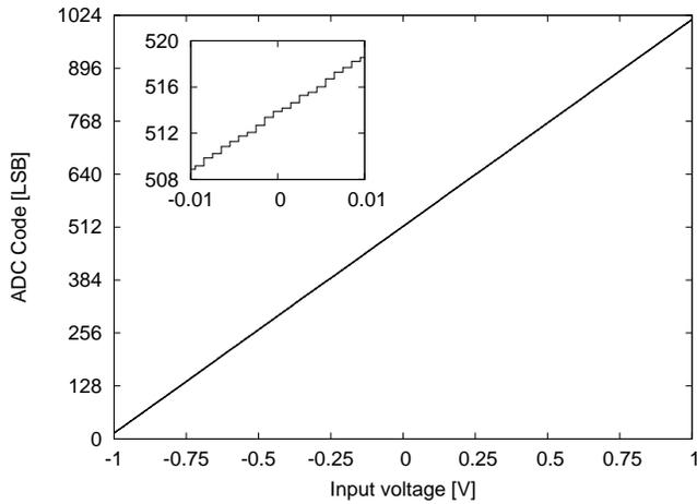
Fig. 8. ADC transfer function measured at 10 MHz sampling frequency.
