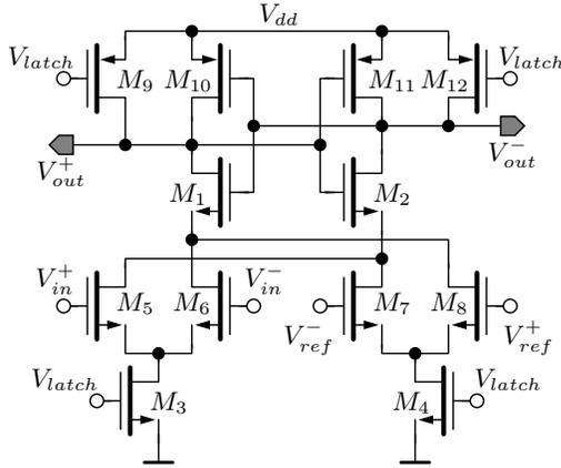
Fig. 5. Block diagram of the dynamic latched comparator.
