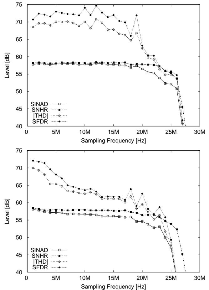
Fig. 11. ADC dynamic performance as a function of sampling rate obtained with input signal signal frequency 1/10th of sampling frequency (up) and at Nyquist frequency (down).
