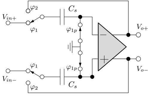
Fig. 2. Simplified schematic of a sample and hold stage. Switches set to sampling phase  $\varphi_1$ .
