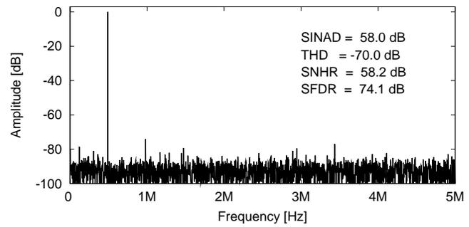
Fig. 10. Example FFT measured for 0.49 MHz input frequency at 10 MHz sampling frequency.
