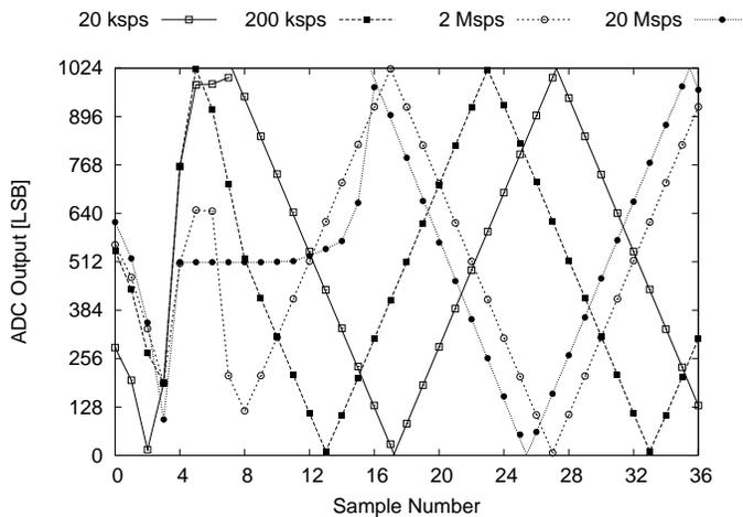
Fig. 15. ADC output versus sample number after power switching on.
