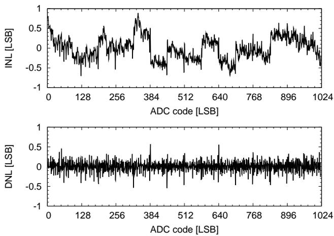
Fig. 9. INL and DNL measured at 10 MHz sampling frequency and calculated using the histogramming method.
