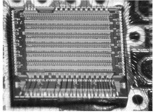
Fig. 7. Photograph of glued and bonded prototype ASIC.
