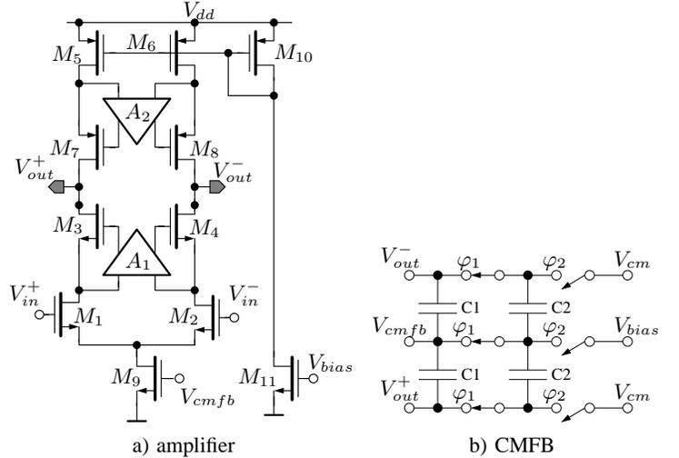
Fig. 4. Block diagram of the fully differential amplifier with boosted gain on the left and SC CMFB circuit on the right.
