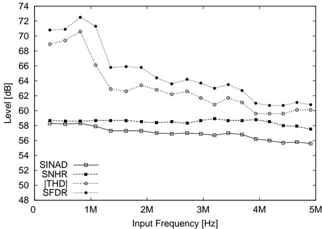
Fig. 12. ADC performance as a function of input signal frequency at 10 MHz sampling frequency.
