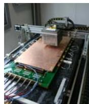
The other detector has been flushed with Ar/CO<sub>2</sub> (70/30) and tested in current-mode with a <sup>137</sup>Cs source (660 keV photons)
