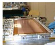
GEM are stretched on a custom-made machine with a tension of ~1kg/cm measured by load-cells
